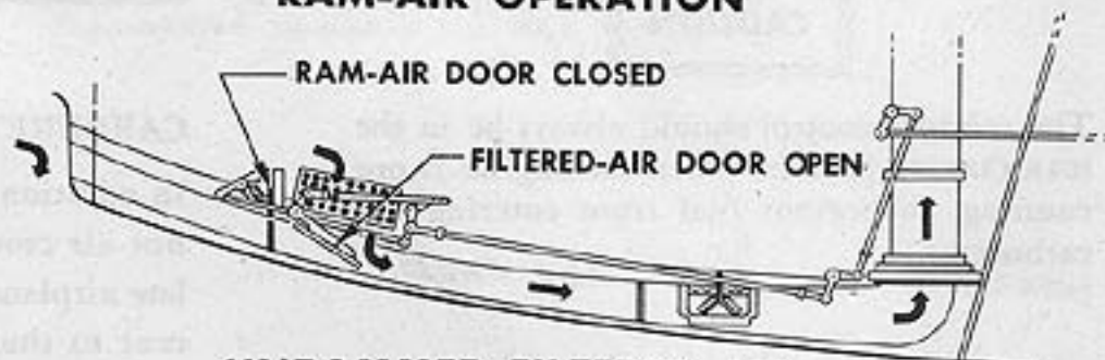
UNRAMMED FILTERED AIR
